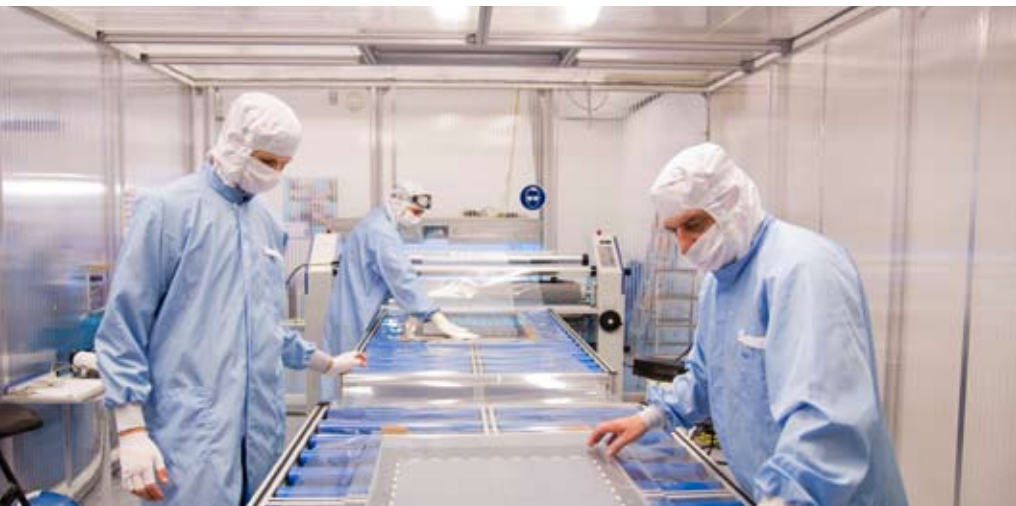
PLEXIGLAS® sheets and films are bonded in a special clean room to avoid any contamination.
